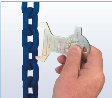
Inspection of permanent elongation
