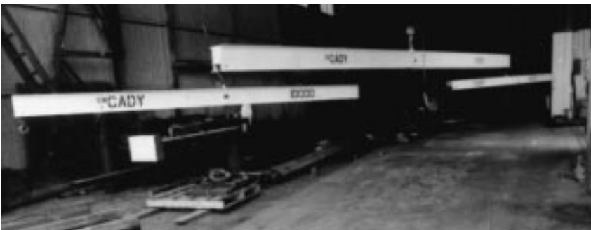
Multiple beam assembly for 60' loads
