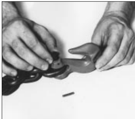
5. Drop load pin into pinhole of the hook.
