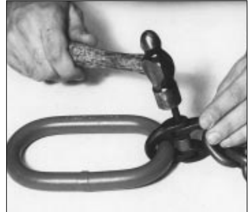
3. Drive the load pin in until the end of the pin is flush with the surface of the body forging.
