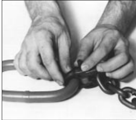
2. Place the stud assembly and the special load pin made from hardened alloy steel in place as shown.
