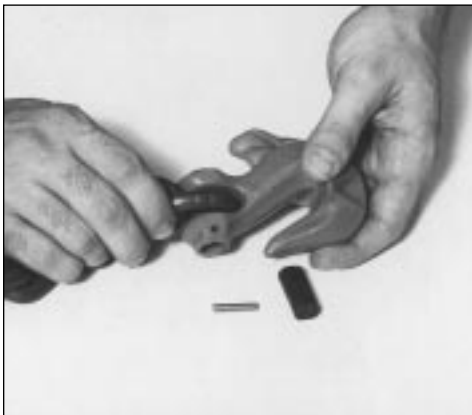
4. Place chain link in clevis slot.
