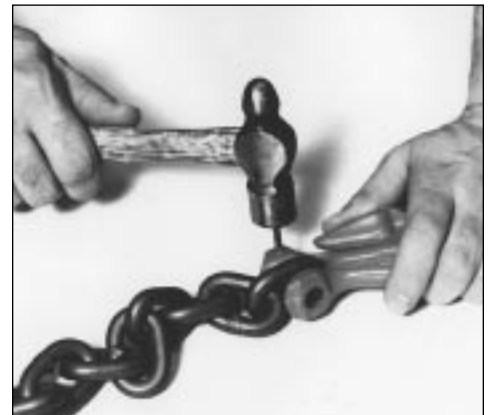
6. Drive single retaining pin until it is flush with the surface of the body forging.
