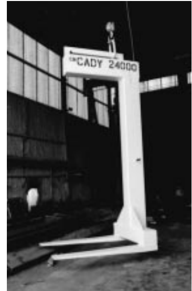
Fixed fork pallet lifter with multi-position bail
