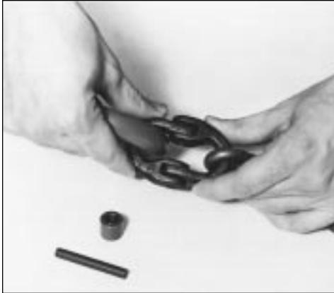
1. Bring the two Hammerlok coupling link body halves together as shown.
