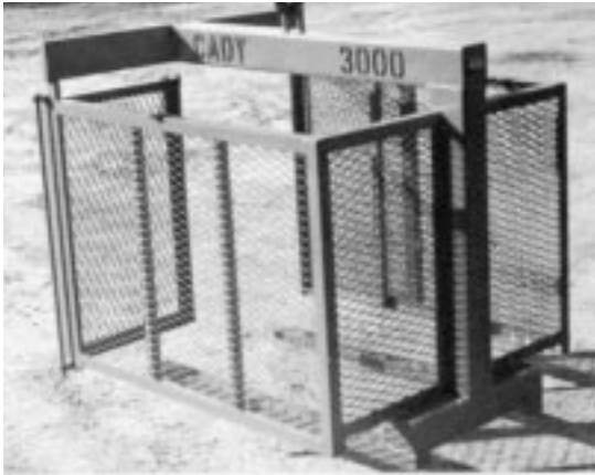
Caged pallet lifter for dangerous loads
