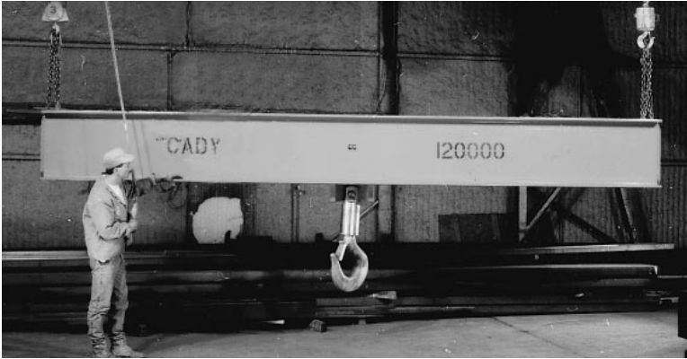
60 ton two hoist beam with roller bearing swivel hook
